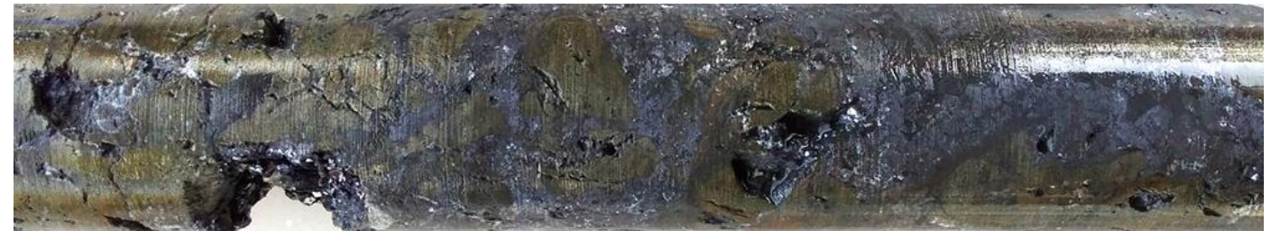
Image: Massive sulphides – Typical galena (grey-blue) with pyrite (bronze colour), diamond core from drill hole AF005 (Phase I extensional drilling). Intersection 11.7m at 10.8% Pb, 105 g/t Ag and 0.4% Zn from 75.7m 1 .
