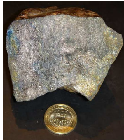
Stream bolder sample of massive pyrrhotite with secondary bornite and chalcocopyrite from Urrao
