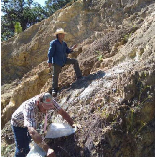
Figure 3: Verification channel sampling at Coaxtlahuacan, over copper-gold mineralised zone. Observed malachite and chalcocite
