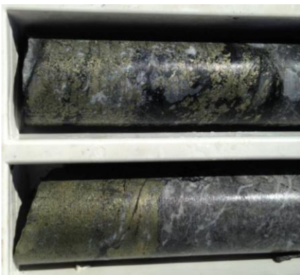
Image: Drill core CCD003 – semi-massive chalcopyrite bands.
