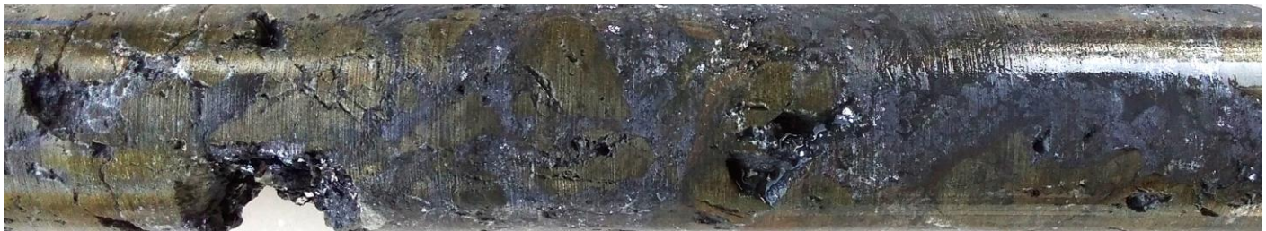
Figure 2: Massive sulphides – Typical galena (grey-blue) with pyrite (bronze colour), diamond core from AF005, 82.1m. Strong lead mineralisation is intersected over 9.4m length in this particular hole.
