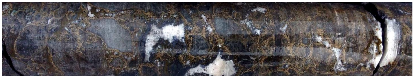
Figure 3: Diamond core from AF013, 124.0m. Example of abundant sphalerite (pale brown) in matrix of dolomite breccia occurs over 4 metres
