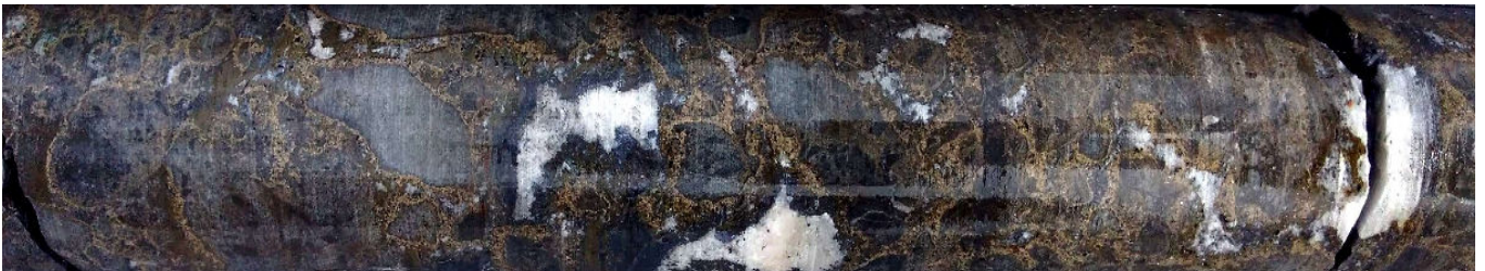
Figure 4. Diamond Core from AF013, 124.0m. Example of Abundant Sphalerite (Pale Brown) in Matrix of Dolomite Breccia Occurs Over 4 Metres
