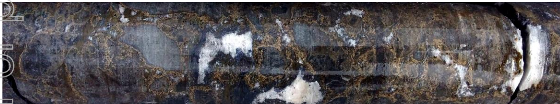
Image: Diamond Core From AF013, 124.0m. Example of Abundant Sphalerite (Pale Brown) in Matrix of Dolomite Breccia Occurs Over 4m 1 .
