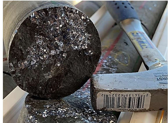
Figure 3: Crystalline Dark Grey Galena in AB034 56.4m (Freshly Broken Core). Part of an interval 52.1m to 59.6m interval with strong galena hosted by slump breccia and Knox Sediments
