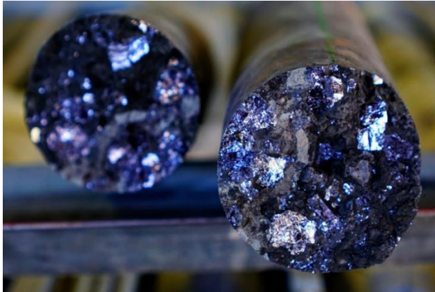
Figure 2: Crystalline Galena in ACD080 32.8m (Freshly Broken Core). Part of an Interval 25.7m to 37.9m of Well Mineralised Core – Consisting of Strong Galena, Some Pyrite and Minor Sphalerite.
