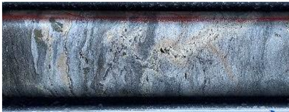
Figure 5: Abundant Cream Coloured Sphalerite in ACD63, 76.7m. Part of an Interval 75.3m to 79.1m With Common Sphalerite as Veins and Matrix Fill in Slump Breccia.
