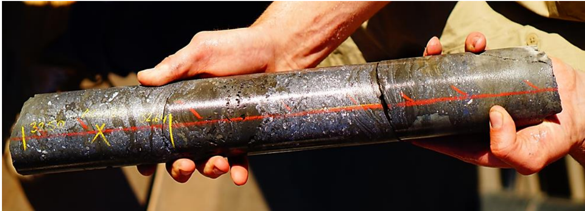
Figure 1: Semi Massive Galena (Grey, Metallic) Replacement. ACD080, 32.8m. Part of an Interval 25.7m to 37.9m (12.2m Length) of Well Mineralised Core – Consisting of Strong Galena, Some Pyrite and Minor Sphalerite.
