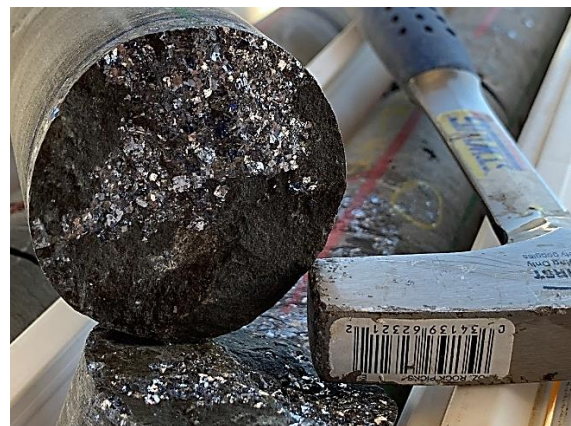
Figure 3: Crystalline Dark Grey Galena in AB034 56.4m (Freshly Broken Core). Part of an Interval 52.1m to 59.6m With Strong Galena Hosted by Slump Breccia and Knox Sediments.
