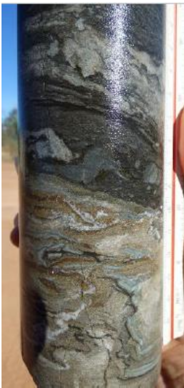
Figure 1: Replacement of evaporite by zinc lead mineralisation.
