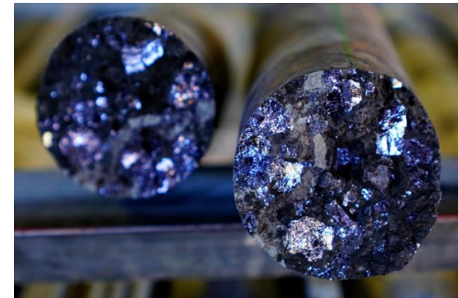
Image 3 : Crystalline Galena in ACD080 32.8m (Freshly Broken Core). Part of an Interval 25.7m to 37.9m of Well Mineralised Core Consisting of Strong Galena, Some Pyrite and Minor Sphalerite.
