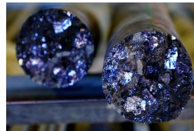
Image 3 : Crystalline Galena in ACD080 32.8m (Freshly Broken Core). Part of an Interval 25.7m to 37.9m of Well Mineralised Core Consisting of Strong Galena, Some Pyrite and Minor Sphalerite.
