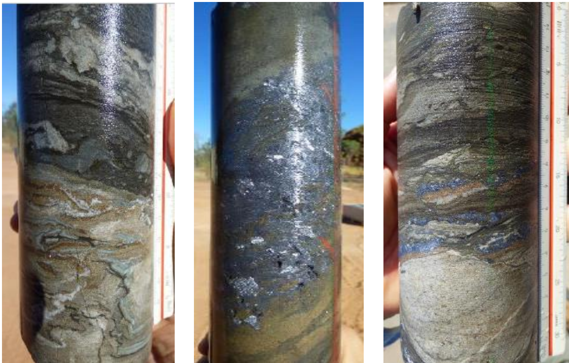
Figure 2: (From left to right) Replacement of evaporite by zinc-lead mineralisation, Galena (lead-sulphide) dominant mineralisation replacing matrix of stratiform breccia, and, Deformed stratiform zinc-lead mineralisation in the Sorby breccia (galena blue-grey and sphalerite pale brown).
