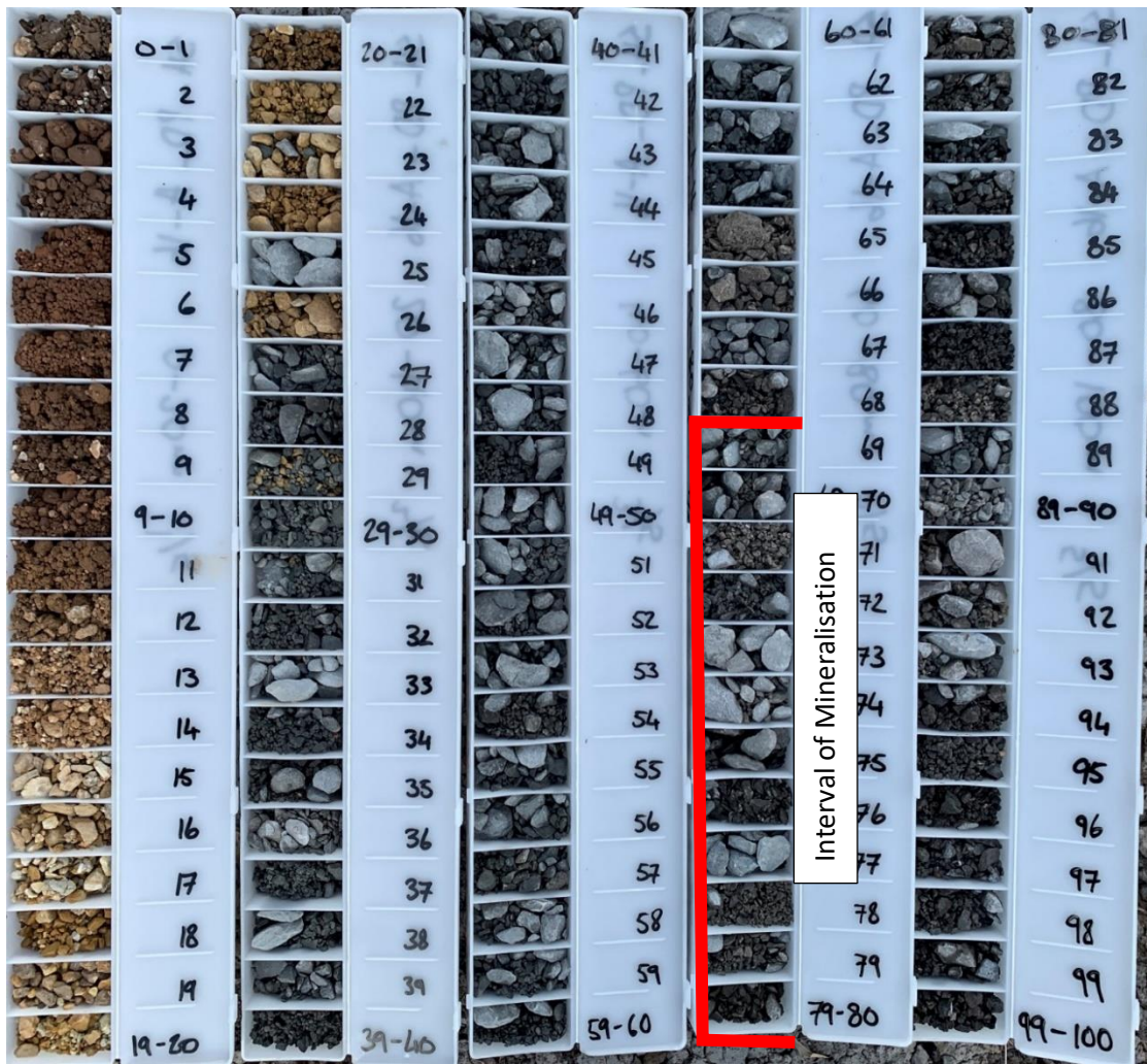
Figure 1. Complete chip trays for RC drill hole SH_PD_A_16 drilled from surface as part of the south-eastern Omega extension targets. Chip trays highlight alluvial clays (0-12 m), supergene alteration zone (12-26 m) and fresh rock from 26 m to the end of hole at 100 m. The highlighted interval (red) from 68-80 represents a mineralised interval hosted in dolomitic grainstones, shaley dolomites and silty dolomites. Chips from 76-77 m contain abundant galena visible as pale silver surfaces (crystals) against the pale grey silty-dolomite host.
