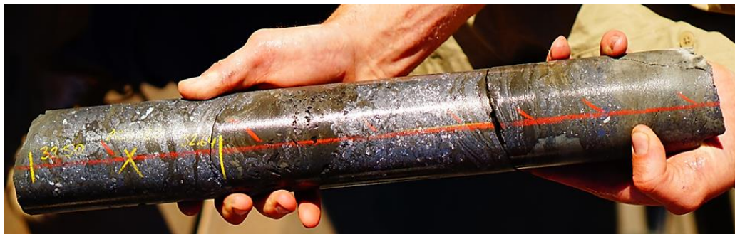
Figure 3: Semi Massive Galena (Grey, Metallic) Replacement. ACD080, 32.8m.
