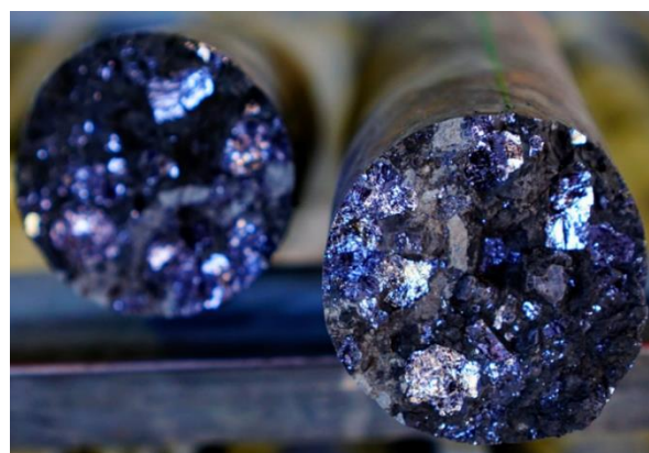
Figure 4: Crystalline Galena in ACD080 32.8m (Freshly Broken Core). Part of an Interval 25.7m to 37.9m of Well Mineralised Core – Consisting of Strong Galena, Some Pyrite and Minor Sphalerite.
