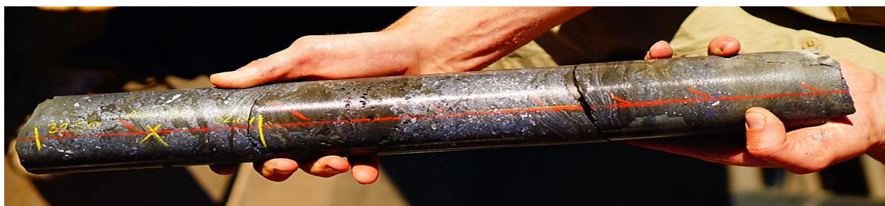
Image: Semi massive galena replacement. ACD080, 32.8m. Part of an interval 25.7m to 37.9m (12.2m) of well mineralised core consisting of strong galena (metallic grey), some pyrite and minor sphalerite.
