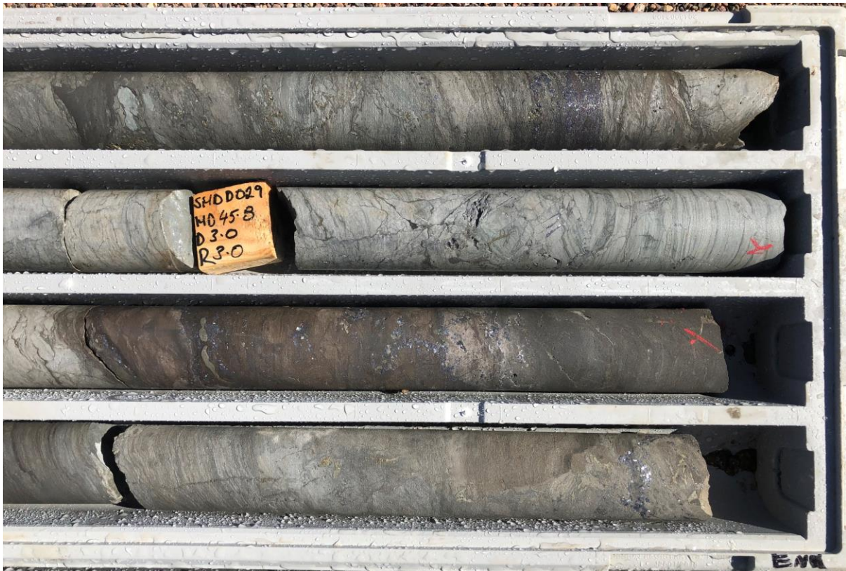
Figure 5: Intra-formational slump breccia and stratabound mineralisation zone intersected in SHDD029 approximately 40m down hole.
