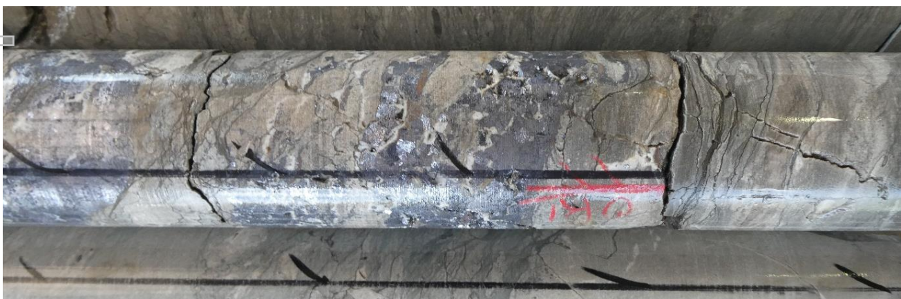
Figure 4: Example of stratiform galena mineralisation interval intersected in SHDD043 at approximately 68m down hole.
