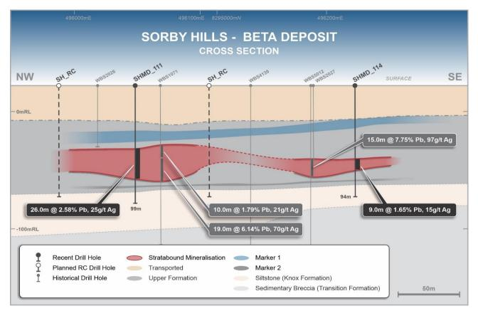
Figure 3 – NW-SE section through the Beta Deposit showing the geometry of mineralisation and location of the new drill intercepts.
