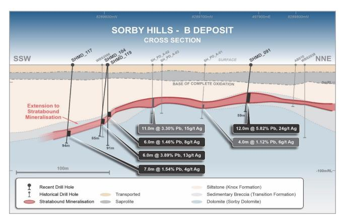
Figure 2 – NNE-SSW section through the B Deposit showing the geometry the mineralisation and location of the new drill intercepts.
