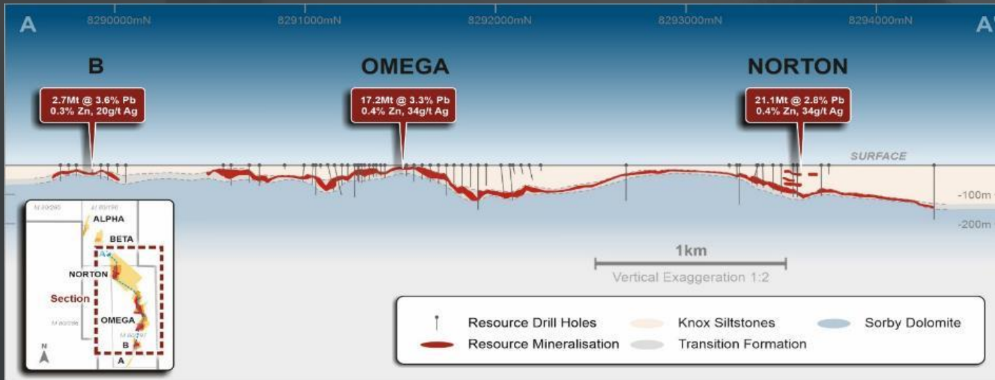
Image: Long section looking west through the Sorby Hills Resource
