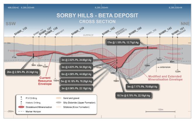
Figure 2 - Beta Cross Section trending NNE (see Figure 1) with incorporation of the latest geological logging and mineralisation observations.
