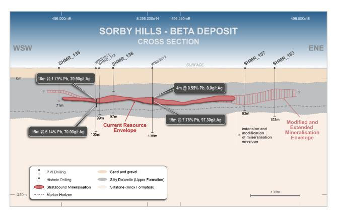
Figure 3 - Beta Cross Section trending ENE (see Figure 1) with incorporation of latest interpretation of geological logging and mineralisation observations.
