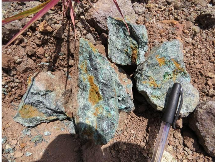
Figure 2: Diorite porphyry containing malachite along a road cut at the Natagaima property
