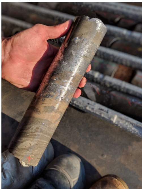
Fig 2: Drill core from infill program. Note coarse galena mineralisation.
