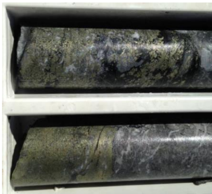
Image: Drill core CCD003 – semi-massive chalcopyrite bands.
