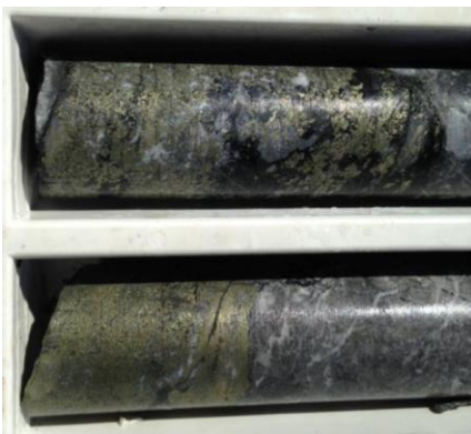
Image: Drill Core CCD03 Semi-Massive Chalcopyrite Bands
