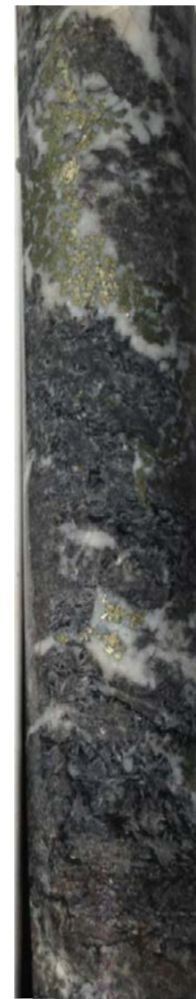
Drill core CCD02, mineralised evaporite horizon, disseminated chalcopyrite. Visible ex-gypsum crystals of evaporite horizon
