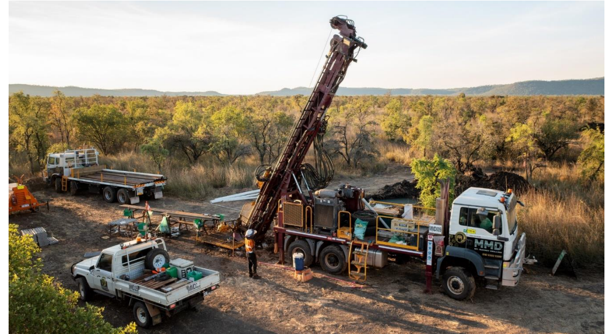
Diamond drill-rig on site undertaking the Phase V drilling program
