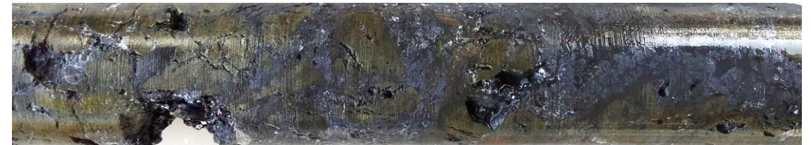
Image: Massive Sulphides – Typical Galena (Grey-Blue) With Pyrite (Bronze Colour), Diamond Core from AF005, 82.1m. Strong Lead Mineralisation is Intersected over 9.4m Length in this Particular Hole 1 .
