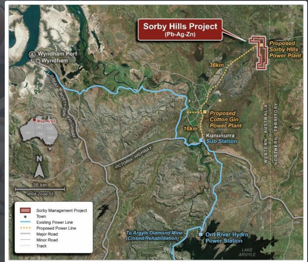
Figure: Location of the Ord River Hydro Power station and existing / proposed transmission infrastructure relative to Sorby Hills
