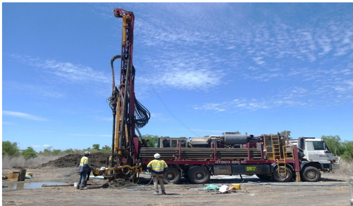
Figure 2: RC Drilling (Phase VI) at Sorby Hills.
