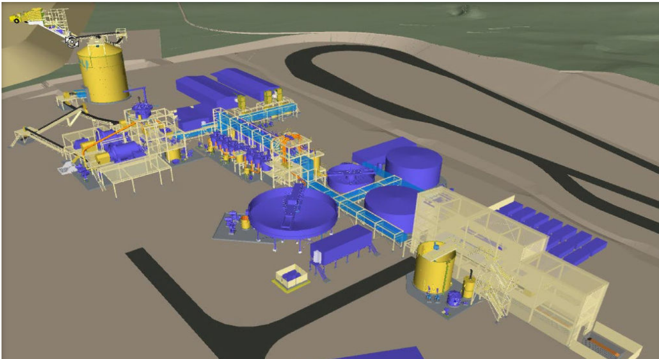
Figure 3: 3D Model of the Sorby Hills Process Plant layout looking northward from the ROM Pad toward the processing facilities and administration buildings.
