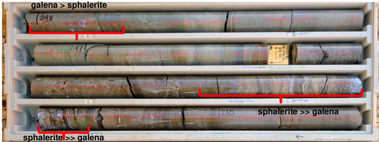
Figure 5 -Photograph of SHSD_185 drill core interval 244.6m to 248.04m showing massive sphalerite + galena replacement mineralisation intervals hosted in bedded carbonates of the Burt Range Basin.
