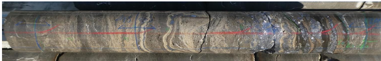
Figure 6 Close up photograph of SHSD_185 drill core interval 245.3m to 246.1m showing colloform massive sulphides (low-iron sphalerite = cream coloured & galena = blue grey)
