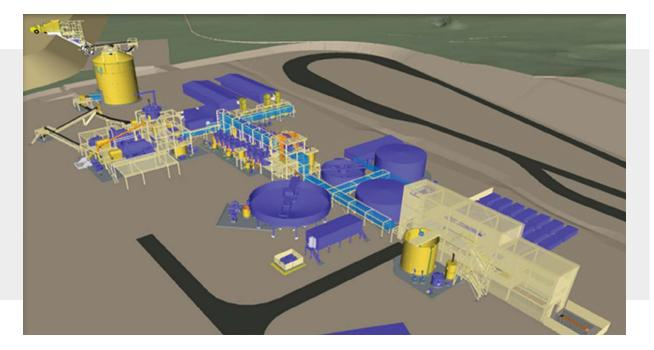
Figure 5: 3D Model of the Sorby Hills Process Plant layout looking northward from the ROM Pad toward the processing facilities and administration buildings.
