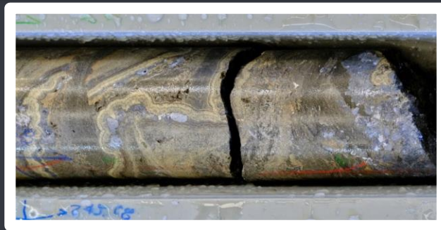
Figures: Section of Keep Seismic Target showing basin margin faults and favourable stratigraphic horizon. Massive replacement style sphalerite (ZnS) and galena (PbS)
