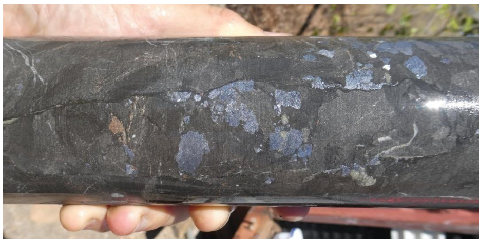
Figure 5 - Photograph of HQ size (6.5 cm diameter) drill core interval from 314.9.3 m to 315.4 m showing massive sphalerite + galena mineralisation intervals.
